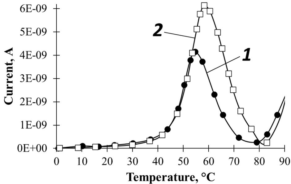
Fig. 4. TSC in P(VDF-TFE) copolymer films polarized at room temperature, depending on the linear heating rate (heating temperature after polarization is 80 °C): 1—linear heating rate  $\beta = 6$  °C/min; 2—linear heating rate  $\beta = 9$  °C/min
