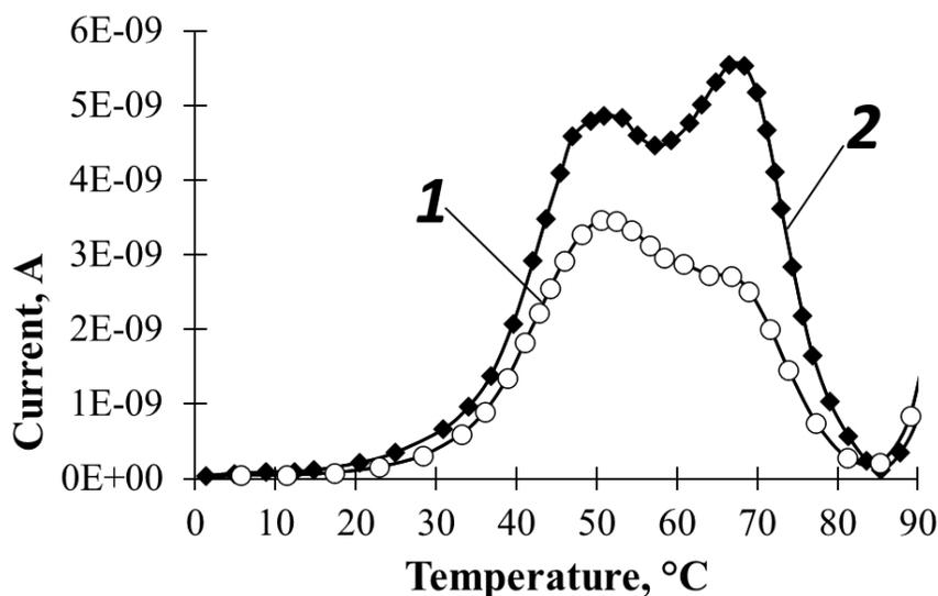
Fig. 1. TSC in P(VDF-TFE) films polarized in the field of a negative corona discharge at different linear heating rates (polarization temperature 80  $^{\circ}\text{C}$ ): 1—linear heating rate  $\beta = 6$   $^{\circ}\text{C}/\text{min}$ ; 2—linear heating rate  $\beta = 9$   $^{\circ}\text{C}/\text{min}$
