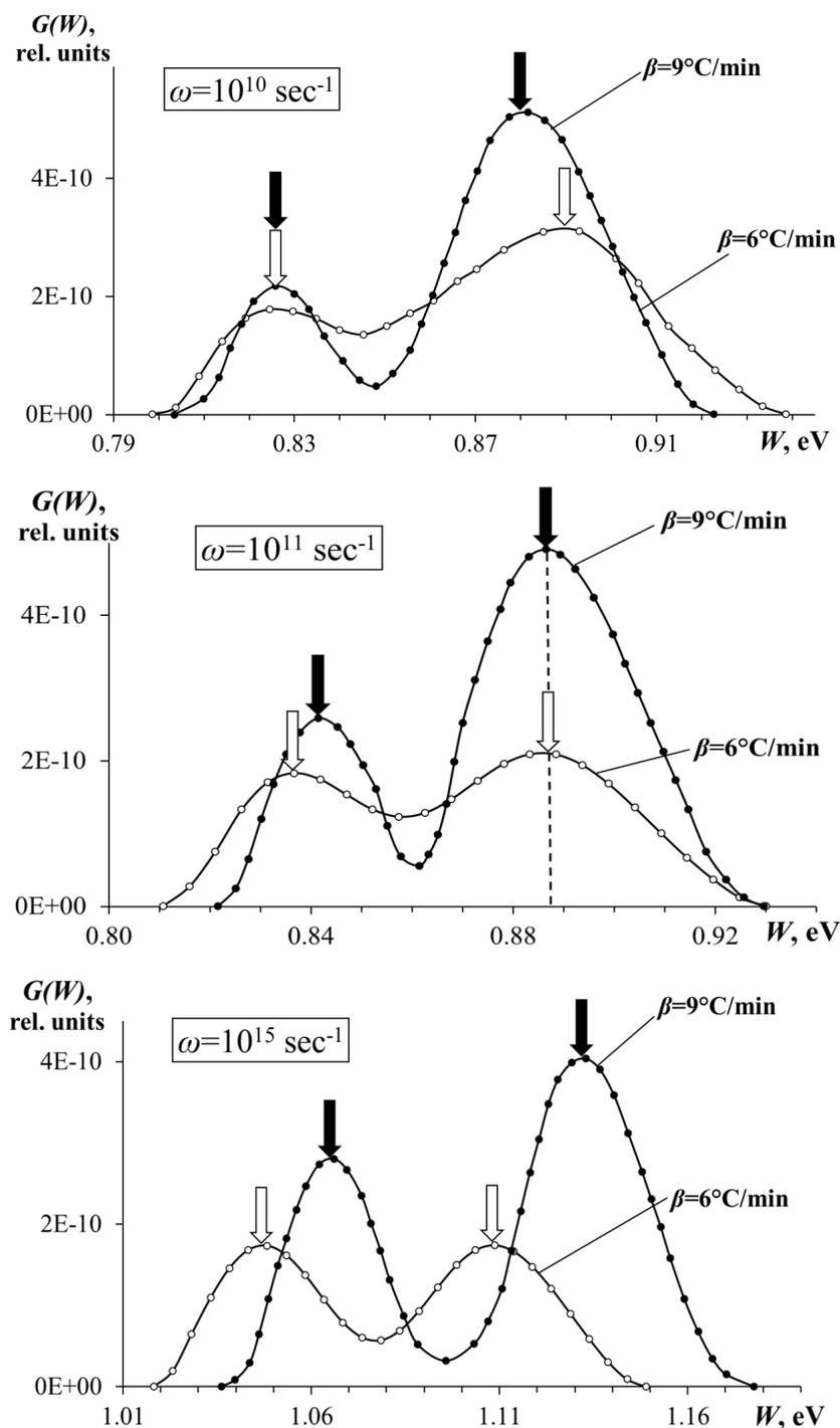
Fig. 3. Versions of the activation energy distribution functions  $G(W)$  for the P(VDF-TFE) copolymer polarized at a temperature of 80 °C in the field of a negative corona discharge for different linear heating rates. Calculation of activation energy and frequency factor for polar structures with higher activation energy
