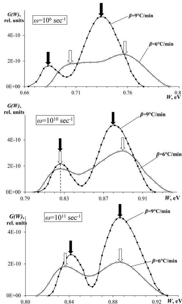
Fig. 2. Versions of the activation energy distribution functions  $G(W)$  for the P(VDF-TFE) copolymer polarized at a temperature of 80 °C in the field of a negative corona discharge for different linear heating rates. Calculation of activation energy and frequency factor for polar structures with lower activation energy
