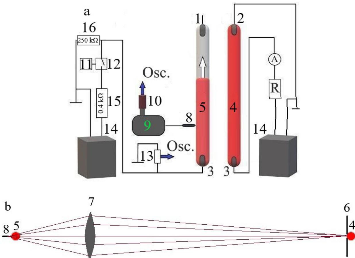
Fig. 1. a — schematic diagram of the experimental setup; b — optical scheme. 1 — unconnected electrode, 2 — grounded electrode, 3 — high voltage electrodes, 4 — radiating tube, 5 — absorbing tube, 6 — diaphragm, 7 — lens, 8 — optical fiber, 9 — monochromator, 10 — PMT, 11 — pulse generator, 12 — switch, 13 — compensated high voltage divider, 14 — high voltage power supply, 15 — resistor (0.4 k $\Omega$ ), 16 — resistor (0.25 M $\Omega$ )
