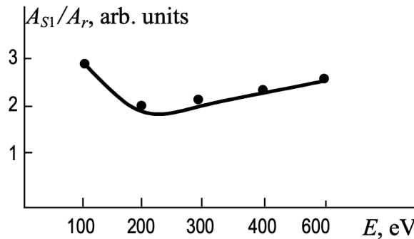
Fig. 6. Dependence of ratio of first surface plasmon intensity to EREP intensity from primary electron energy for Mg. \phi = \alpha = 80^\circ . The solid curve corresponds to the experiment, points correspond to the calculations.
